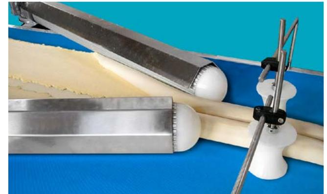
Double rolling dough for automatic and fast production for instance of cinnamon rolls.
