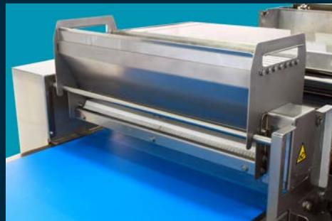
A roller device grants an even, adjustable, sprinkling of flour or sugar. The of stainless steel hopper is easy to remove and easy to clean.
