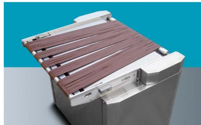
The spreading device is used to spread the strips of dough and can be adjusted by hand.
