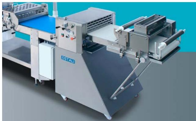
Installed at the entrance of the table, it grants an even thickness of the dough for precise processing, constant weight, etc.
