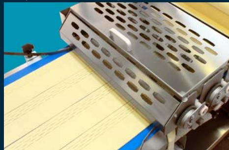
The table is pre-set for the installation of two rotating cutting dies, with total safety protection, to cut/mark/decorate the dough.
