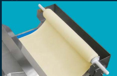
Made of stainless steel, installed on a mobile support with easy fastening, it's ideal for a quick and easy positioning of the rolling pin to start the automatic processing of the dough.
