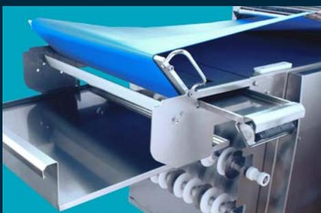
A quick releasing device for belt tension allows easy and careful cleaning of the table with a scraper and the stainless steel removable drawer collects scraps.
