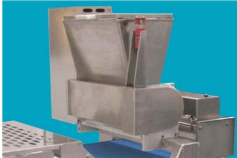
3 rollers extruder to process hard dough gently and for heavy duty use.
